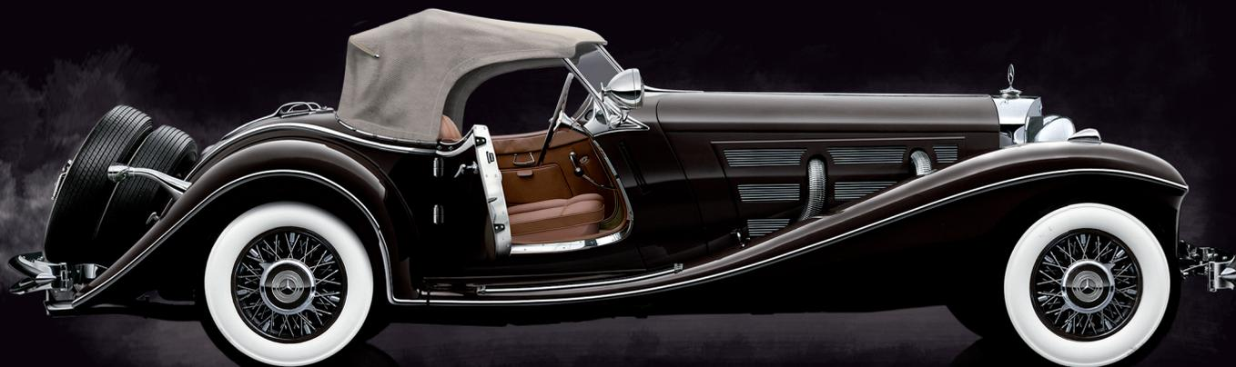
*W*ater-cooled eight-cylinder series motor, camshaft at the side, actuated by spur gears, 100 hp (or 160 hp with actuated dual lobe Roots blower), capacity of 5,018 ccm, maximum speed of 160 km/h, wheelbase of 3,290 mm, front and rear gauge of 1,535/1,547 mm respectively, total length of 5,000 mm, kerb weight of 2,250 kg, consumption of 27 l per 100 km.
